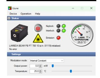
All operating parameters can be monitored and controlled from a PC using the Ltune laser control software for Windows. Alternatively, the laser can easily be controlled from your own application software. Please refer to the user manual for a detailed description of the communication protocol. You can find downloads on our website
