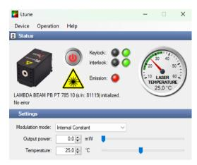
All operating parameters can be monitored and controlled from a PC using the Ltune laser control software for Windows. Alternatively, the laser can easily be controlled from your own application software. Please refer to the user manual for a detailed description of the communication protocol. You can find downloads on our website
